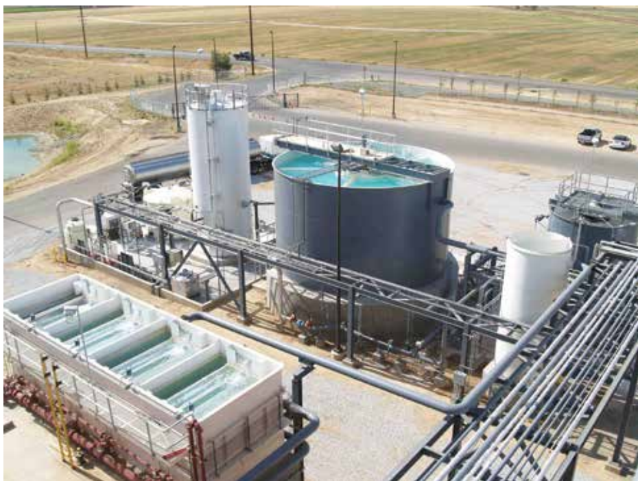
Cold Lime Softening Clarifier at a Western dry grind ethanol facility where a ZLD system was implemented. CLS is this decade's old technology that is making a comeback as it is common in ZLD systems.
